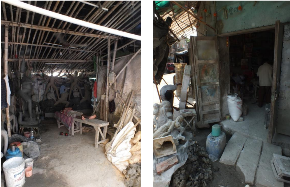
Image 2: Two larger workshops showing (a) internal layout during afternoon break and bamboo-slat roof with polythene insulation and (b) workshop frontage with half- folded shutters, wooden ramp and materials on the street.
